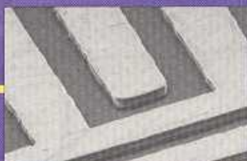
MAGNIFICATION: 1.21KX 5 Micron Conductors 5 Micron Spaces
